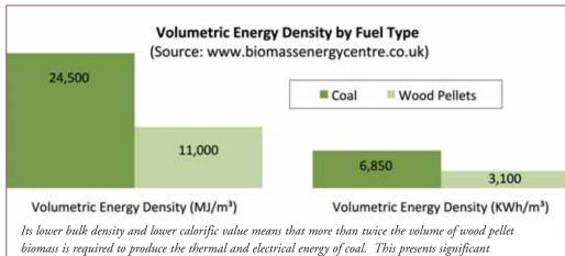
biomass is required to produce the thermal and electrical energy of coal. This presents significant considerations in the design and manufacture of biomass loading chutes.
