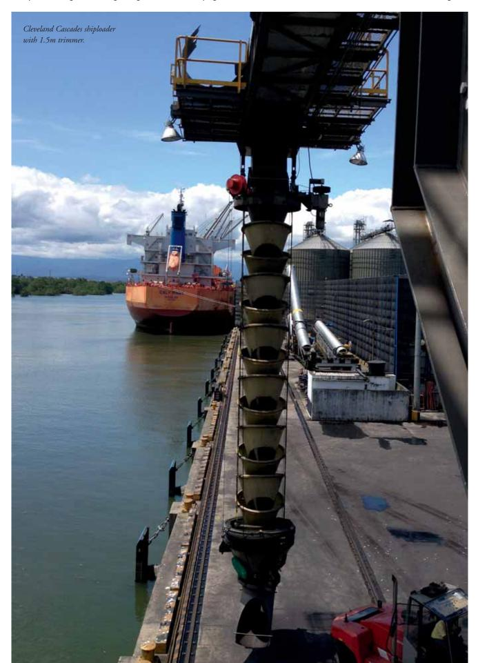
series of oppositely inclined cones, which controls the flow at low velocity, yet high volume. During its descent, the material is supported through the full length of the chute, ensuring a soft delivery from the outlet to the material pile, for every load. It therefore arrives at the load pile with minimal degradation. The controlled descent of the material prevents air separating the particles and largely eliminates dust generation at source.
