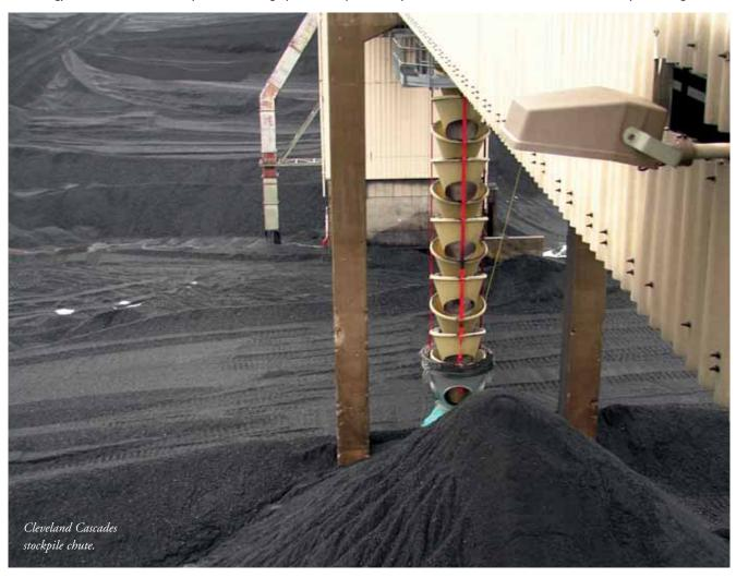
cascade shiploaders, transfer chutes and free fall vehicle loading chutes.
