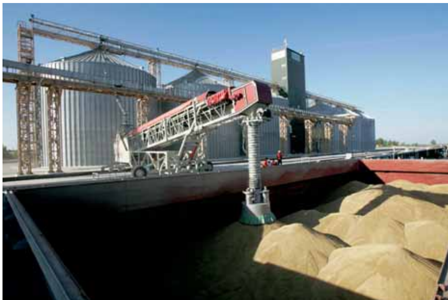
Case Study 3: Grain - Nibulon, Ukraine. Loading mobility is often an issue facing port operators. This photograph shows one of eleven chutes for mobile shiploaders supplied by Cleveland Cascades for grain handling facilities in Ukraine. The lightweight nature of the freefall chute facilitates movement along the full length of the quay. Dust emissions are minimized by high specification extraction units at the base of the chute. This removes the need for heavier dust extraction units on the quayside and reduces material wastage as the dusty material is re-circulated and loaded onto the pile.
