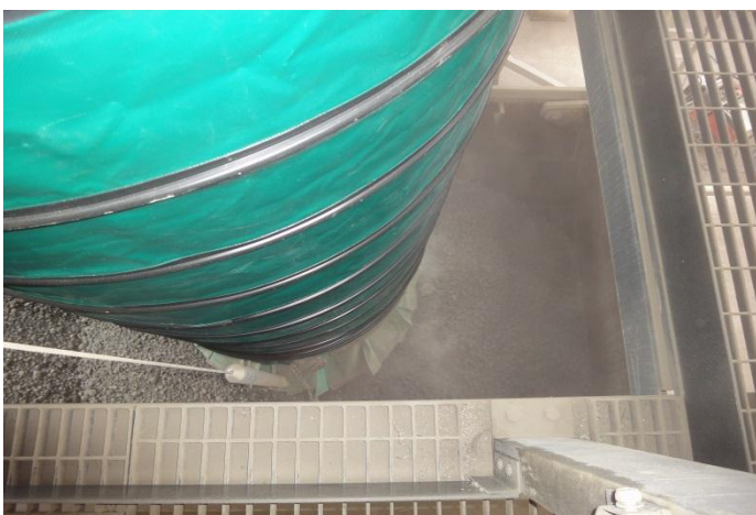
The Vehicle Loading Chutes are used to load Cement Clinker at rates 330tph.
