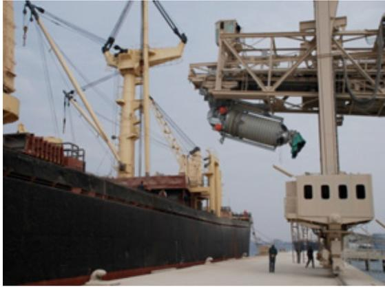
Cleveland Cascade engineers were able to provide a bespoke loading solution to the Port Authorities specific problems. Additionally, Cleveland Cascades undertook project management of the installation and commissioning phases which included integration of the new chute control unit into the existing shiploader control system.
