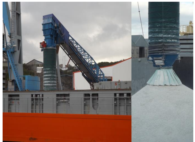
The chute is fitted to a small mobile loader, and utilises our standard skirted outlet for excellent dust control during loading.
