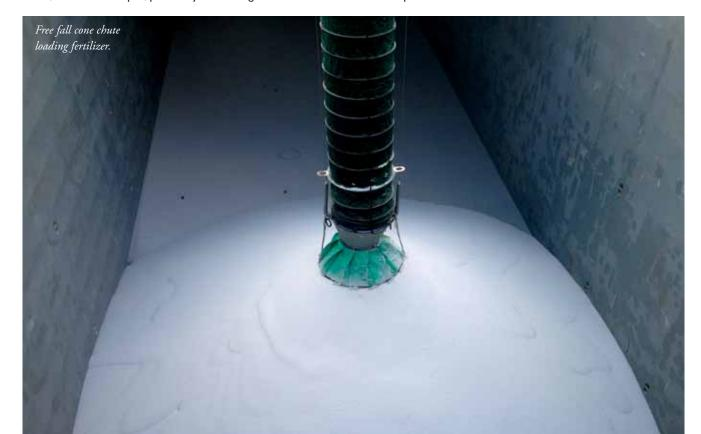
fall chutes. The investment has enabled the launch of both free fall cone and tube chutes. The cone system utilizes a series of vertical cones suspended from chains or strops, allowing the material to fall vertically to the pile. The tube system uses of a series of telescoping concentric tubes which remains rigid and is ideally suited to applications which require trimming spouts or jet slinger devices.
