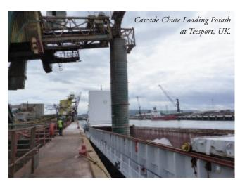
Cascade concept, which utilized a series of inclined cones to control the velocity and flow of their Potash.
