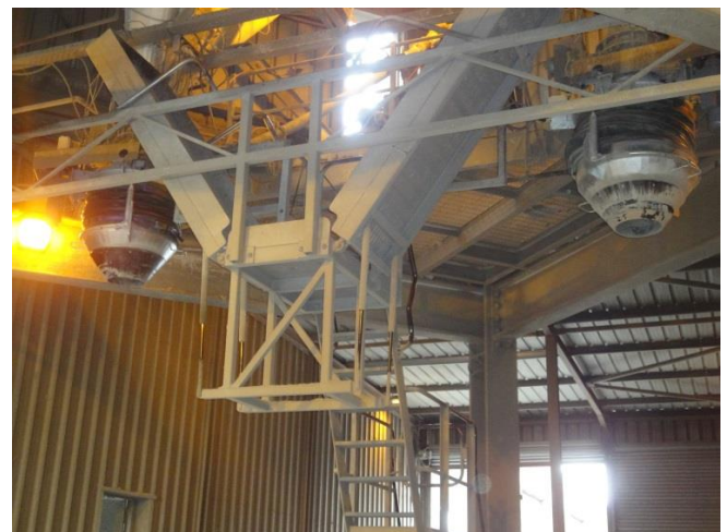
The chute is equipped with a rubber seal at the outlet which sits inside the hatch of the truck. This creates a perfect seal for dust-free loading.
