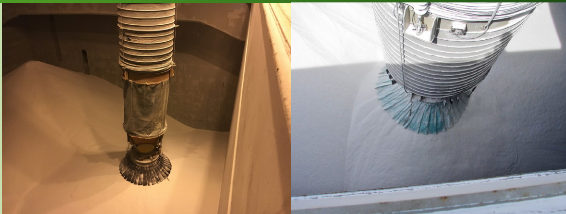
Above left: Cleveland Cascades Ship Loader - Alumina, Brazil Above right: Cleveland Cascades Cascade Shiploader – Alumina, Australia.
