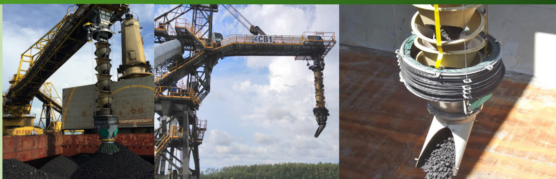
Above left: Cleveland Cascades Ship Loader - Coal, Columbia Above centre & right: Cleveland Cascades Cascade Ship loader with rotating Trimmer Spout- Loading Coal & Coke.
