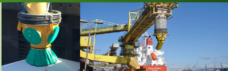
Above left: Cleveland Cascades Shiploader Loading Potash - USA Above Right: Cleveland Cascades Cascade Ship loader – Potash, Germany.
