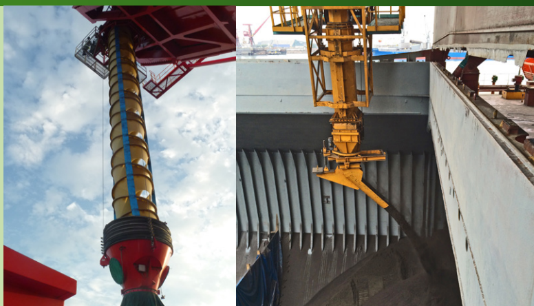
Above left: Cleveland Cascades Ship Loader - South Africa Above right: Cleveland Cascades Free Fall Telescopic Shiploader handling various Concentrates, Peru.
