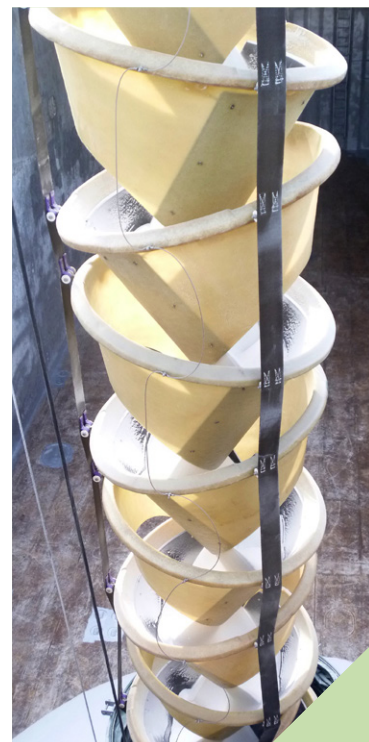
Above: Materials flowing at a controlled speed through the cascade system
