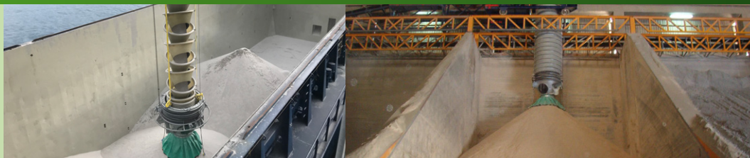
Above Left: Cleveland Cascades Shiploader Loading Nepheline Syenite - Norway Above Right: Cleveland Cascades Cascade Stockpiler – Gypsum loading, Portugal.
