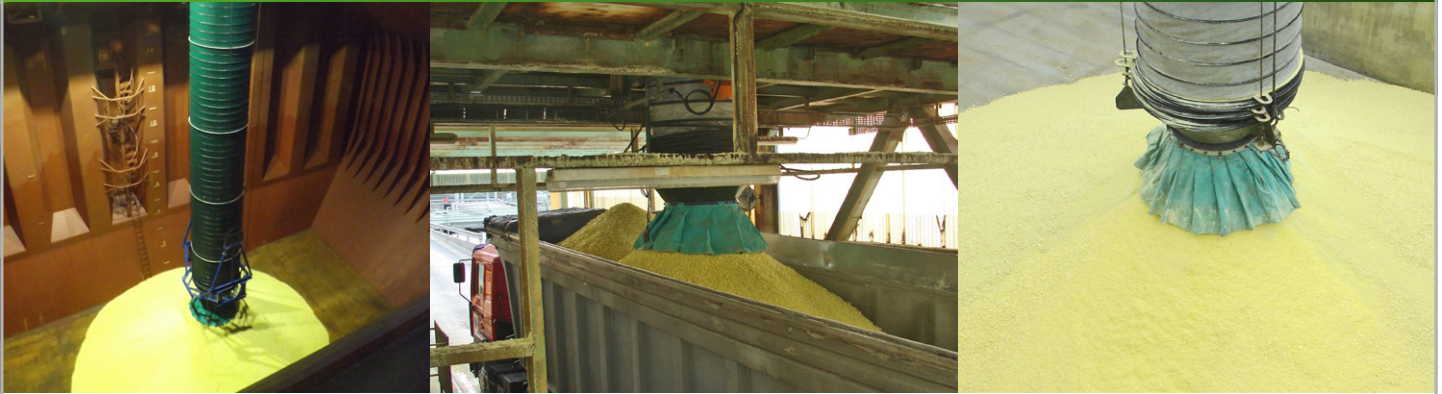
Above left: Cleveland Cascades Ship Loader Loading Sulphur - USA Above centre: Cleveland Cascades Open Truck Loader handling Sulphur Above right: Ship Loader handling Sulphur.
