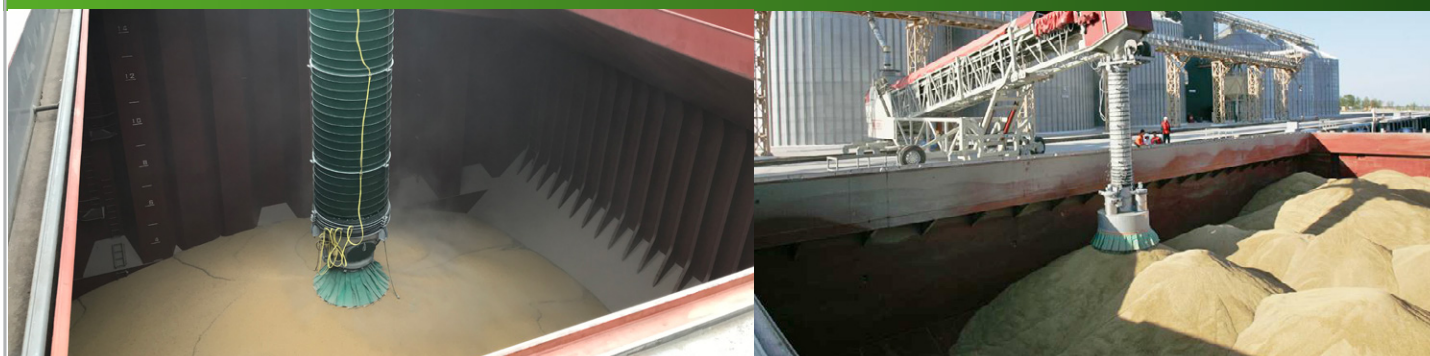
Above left: Cleveland Cascades Ship Loader - Grain, USA Above right: Cleveland Cascades Free Fall Shiploader handling Grain, Ukraine.
